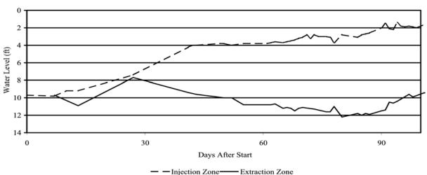
Figure 1 Water Level (Initial operation w/ no bioicide)
